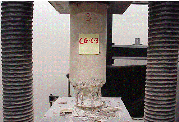
Figure 20 Cast earth column after testing
