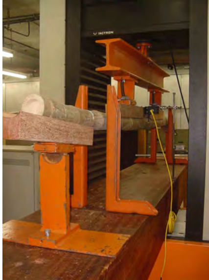
FIGURE 2 – THIRD-POINT LOADING BENDING STRENGTH TEST FOR BAMBOO CULM.
