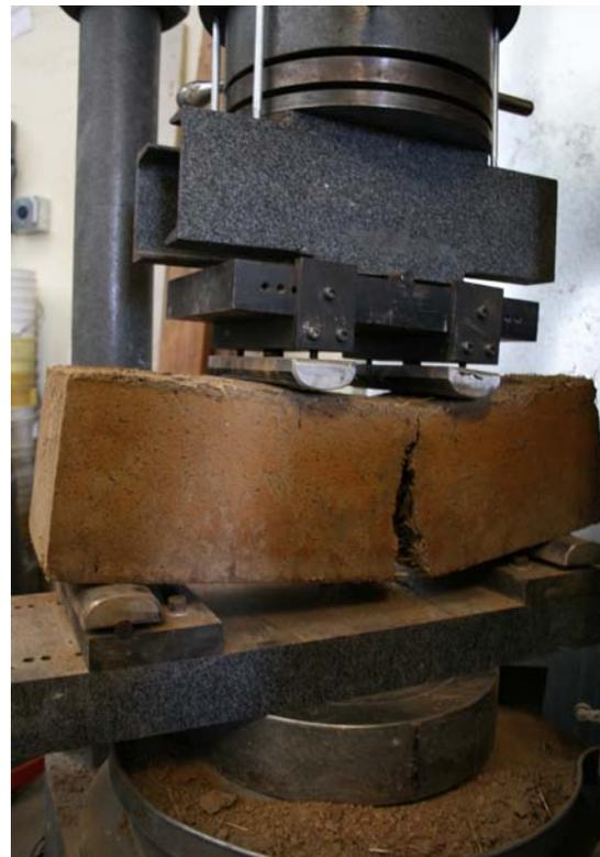
stress at the bottom of the beams at approximately 125 psi/min until failure occurred, defined for this study as severe cracking and at least one inch of vertical deflection. The shrunken dimensions of the beams (prior to loading) were used to calculate the moduli of rupture.
