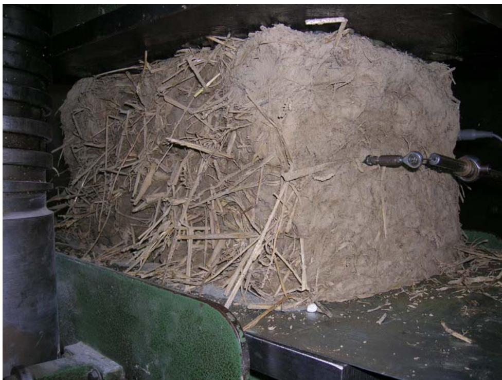
Figure 7. A raw-earth cob sample tested by uniaxial compression.
