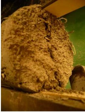
Fig 10. Cylinder tested in splitting tension to determine tensile capacity
