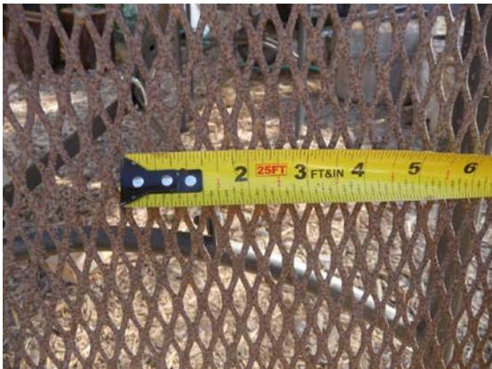
*Fig 3. Wetted soil was sifted through this  $\frac{1}{2}$ " expanded lath screen.*
