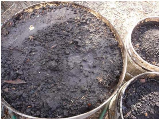
*Fig 1. Dry soil soaking in water at a 1:1 volumetric ratio*
