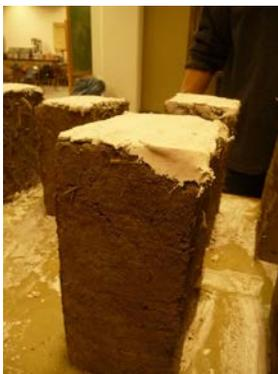
*Fig 7. Caps compensate for uneven geometry*
