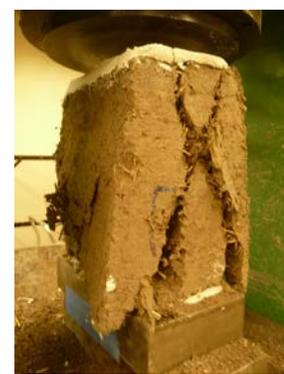
*Fig 9. Prism tested to failure.*
