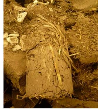
Fig 12. Ductile nature of long-straw cylinders
