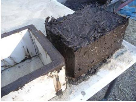
Fig 4. A prism removed from its mold and set to dry.
