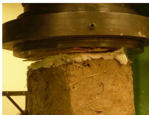
*Fig 8. Wood shims create a more even testing surface under loading cell.*
