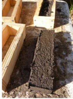
Fig 5. A beam drying next to its mold.
