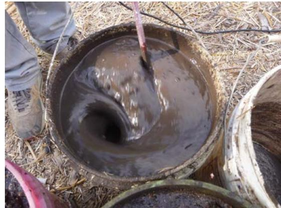
*Fig 2. Creating a homogeneous wetted soil mixture with a paddle extension on a power drill.*
