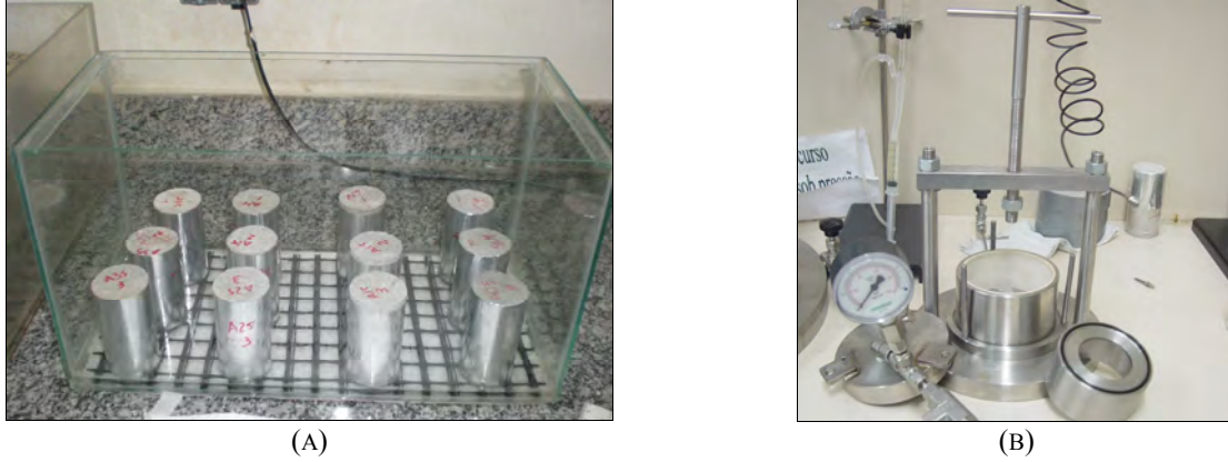
FIGURE 4 – WATER CAPILLARY SORPTION TEST (A) AND GAS PERMEAMETER USED IN THE STUDY (B).
