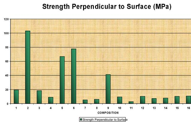
**FIGURE 3. BEHAVIOR OF THE TENSILE STRENGTH PERPENDICULAR TO THE SURFACE VS. COMPOSITION**
