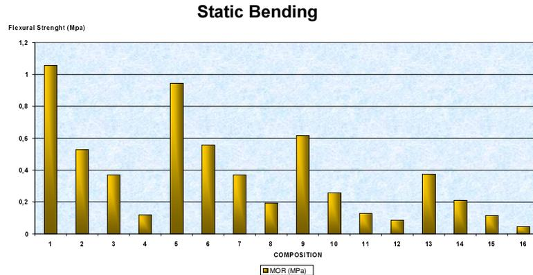
**FIGURA 2.** BEHAVIOR OF THE MODULUS OF RUPTURE VS. COMPOSITION
