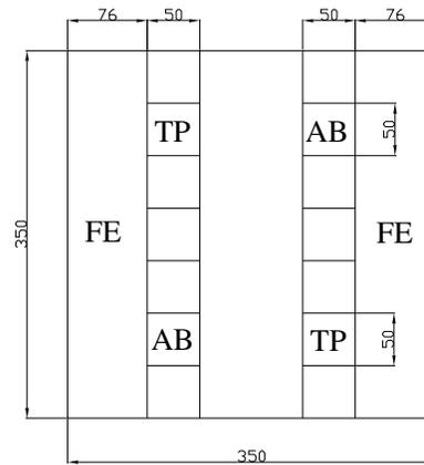
**FIGURE 1. TESTING PANELS** FIGURE (TP-Tensile Perpendicular, AB-Water Absorption, FE- Static Bending)
