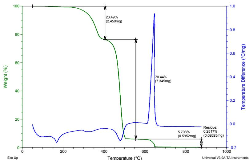
FIGURE 2. THERMOGRAVIMETRY CURVE OF SAMPLE NUMBER 2.
