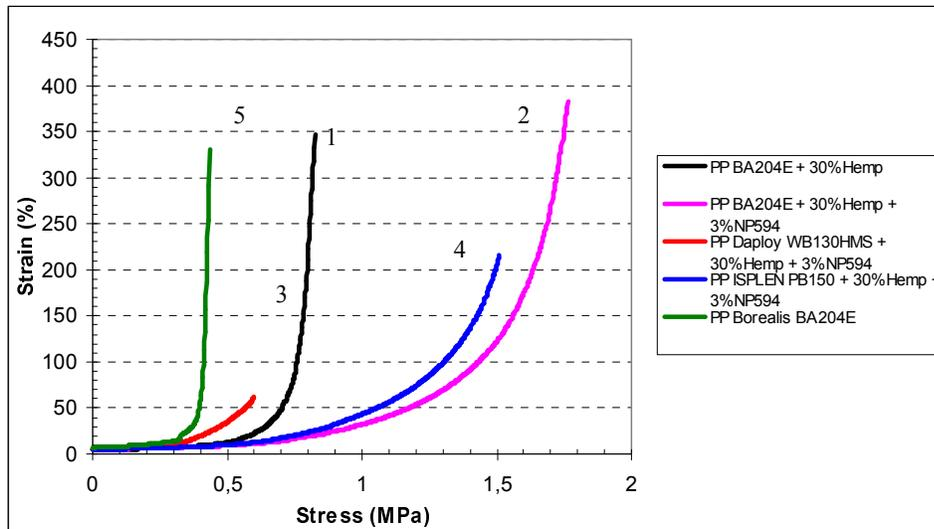
FIGURE 4. STRESS/STRAIN CURVES AT 160°C OF SOME COMPOUNDS OF HEMP-POLYPROPYLENE.
