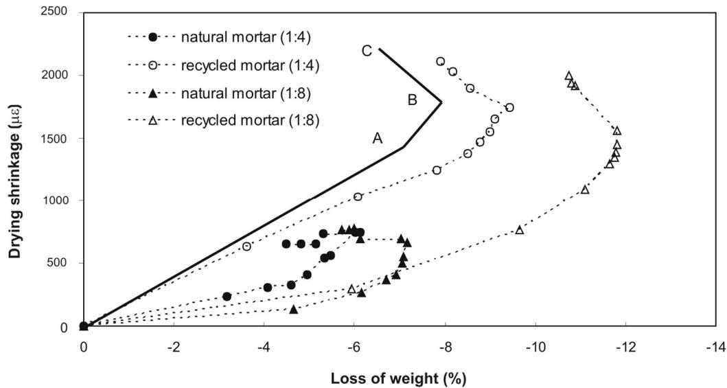
FIGURE 5 –DRYING SHRINKAGE DEFORMATION VS. LOSS OF WEIGHT
