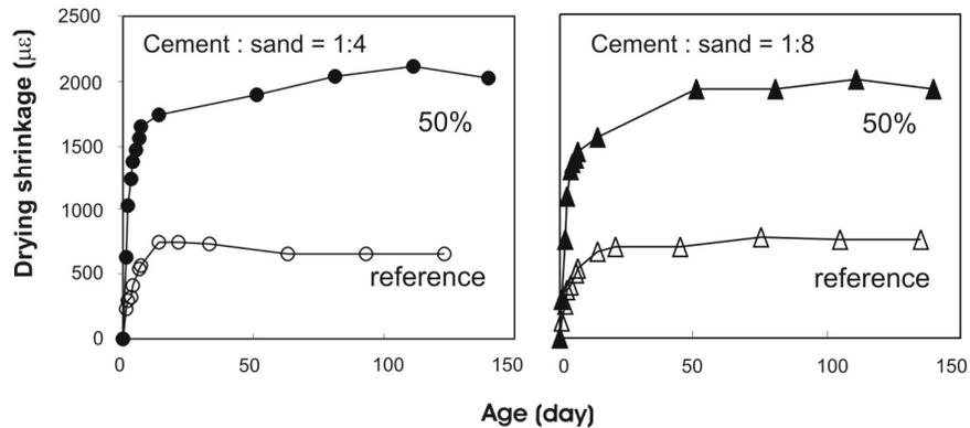
**FIGURE 4 – DRYING SHRINKAGE VS. AGE**
