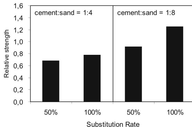
**FIGURE 3 – INFLUENCE OF AGGREGATE SUBSTITUTION RATE ON RECYCLED MORTAR COMPRESSIVE STRENGTH RELATED WITH NATURAL MORTAR COMPRESSIVE STRENGTH**
