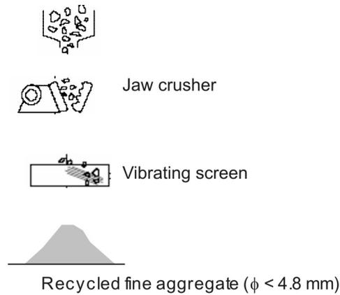
**FIGURE 1 - FLOW CHART OF RECYCLED AGGREGATE PRODUCTION**
