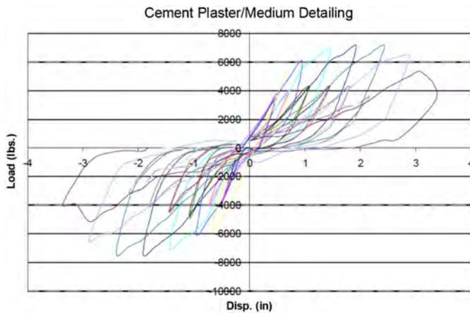
**Fig. 6.** Load-displacement response of slender wall tested by Faurot et al. (2004) (reprinted with permission from authors)
