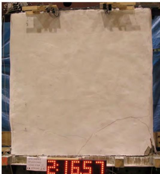
Fig. 4. Flexural cracks in Wall E (2.5% drift level)
