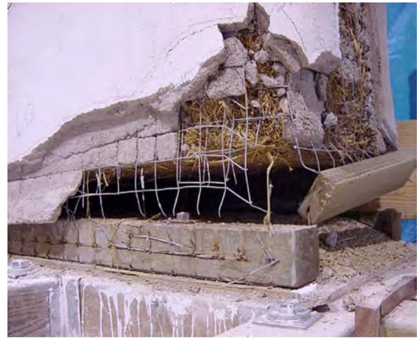
Fig. 5. Wall E mesh failure (7.5% drift level)
