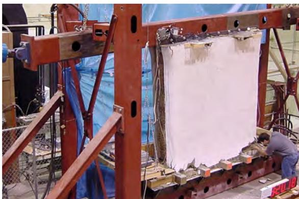
Fig. 1. Overview of full-scale test setup used by Ash et al. (2003)
