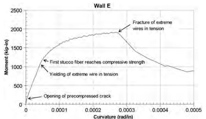
**Fig. 7.** Moment-curvature response for Wall E, computed using *BIAX*
