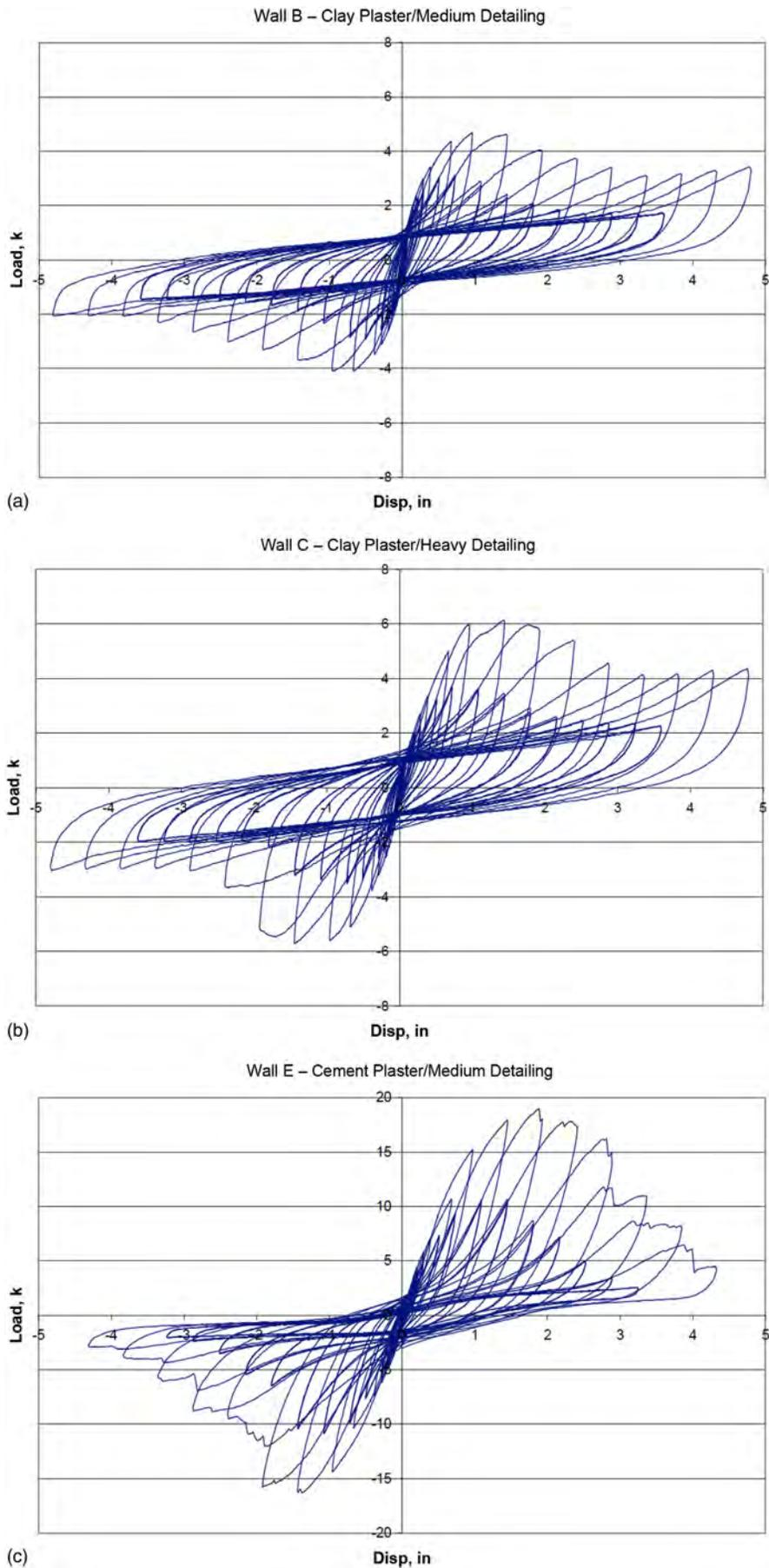
**Fig. 3.** Load-displacement plot for (a) Wall B; (b) Wall C; (c) Wall E
