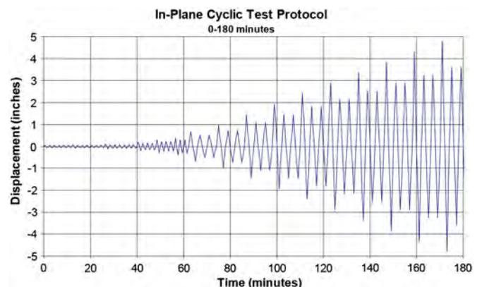
Fig. 2. Reversed cyclic loading protocol to 5% drift (4.92 in.)
